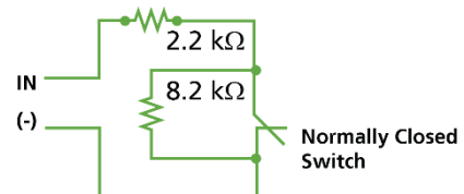
Figure 7: Normally Closed Supervised Input with Double Resistors
