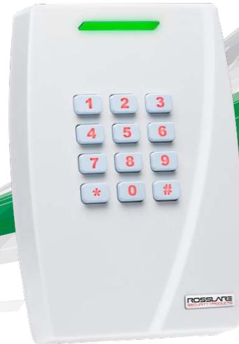
This MIFARE Classic® EV1 13.65MHz Smartcard and PIN code reader has an elegant design with backlit keys. AY-W6350 is an advanced model with multi-format outputs for high compatibility with standard host access controllers. It has a local menu to program facility code as well as Card & PIN credential modes. This fully-potted model resists dust and moisture at level IP65.
