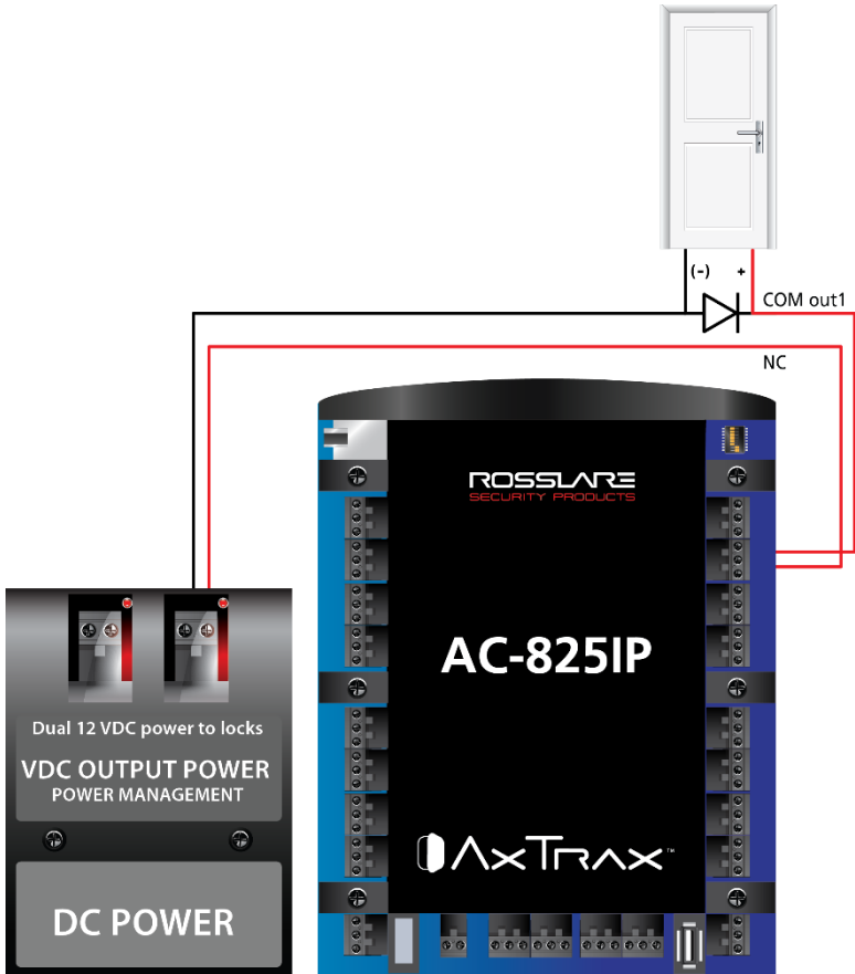
Figure 13: Door Lock – Failed Open
