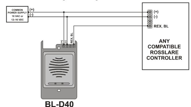
**Note** It is recommended that 22 Gage wire be used between the BL-D40 and the controller.
