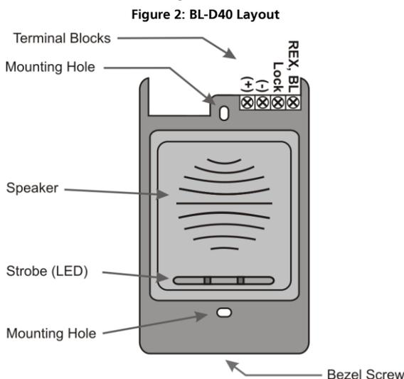
2. Screw the BL-D40 onto a US Gang Box through the two mounting holes provided (Figure 2).
