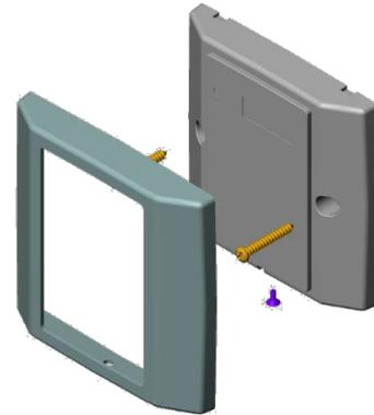
7. Align the two holes of the reader with those drilled in the wall and firmly attach the reader to the wall with two screws, whose size is indicated on the template.
